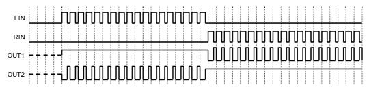
Fig.40 PWM control operation (timing chart)
