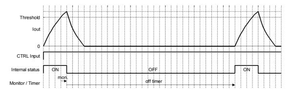
Fig.42 Over current protection (timing chart)
