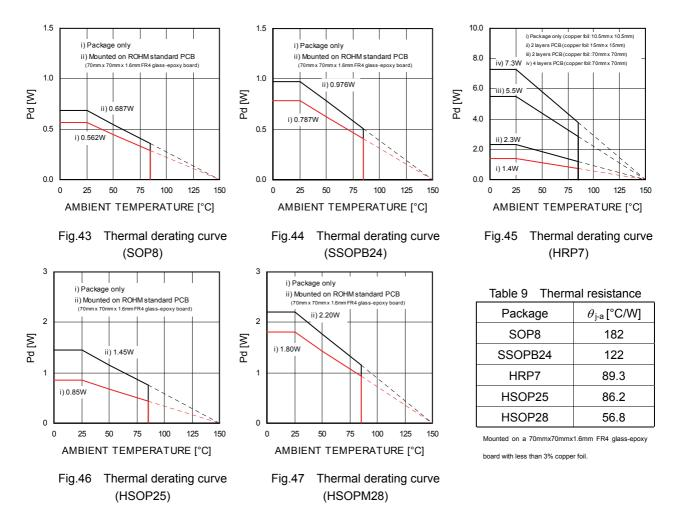
Thermal design needs to meet the following operating conditions.
