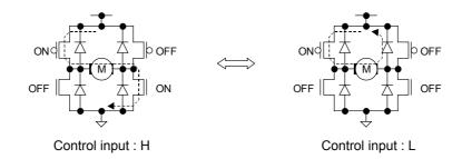
Fig.39 PWM control operation (output stage)
