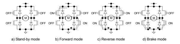
Fig.38 Four basic operations (output stage)
