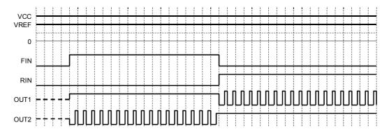
Fig.41 VREF control operation (timing chart)
